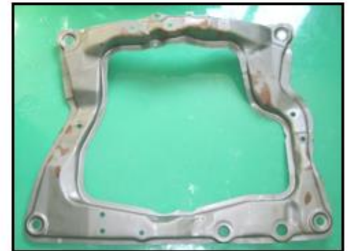
( HMC ) FRT FRAME Material : SPH-270D 1.6 mm
