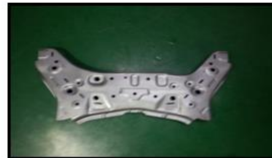
( HMC ) FRT CROSS MBR LWR Material : SGARC440 60/60 1.8 mm
