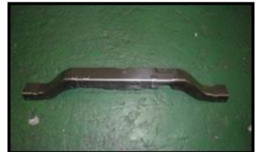
( PROTON ) PANEL FRT END CTR Material : SPCC 1.0 mm
