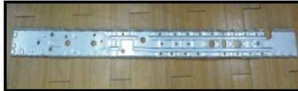
( GM ) REINFORCEMENT-RKR INR PNL LH/RH Material : CR980T/700Y-MP
