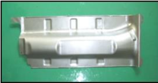
( HMC ) HEAT PROTECTOR Material : SACD 0.6 mm
