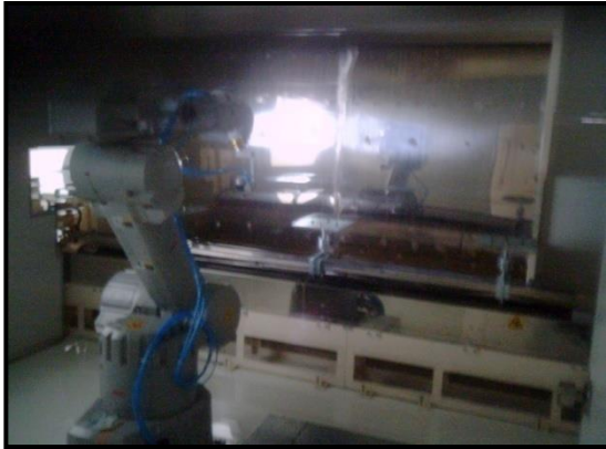
Lamp robot coating system
