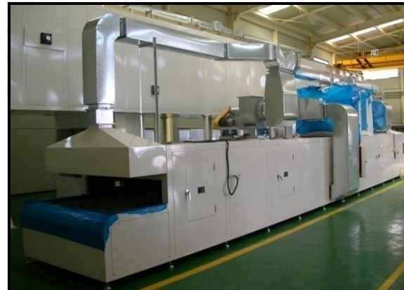
Head lamp UV coating line
