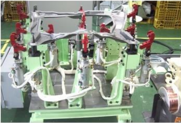
Welding Jig and robot system
