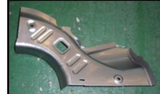
( PROTON ) PANEL REAR END RH Material : SPRC45 0.85mm
