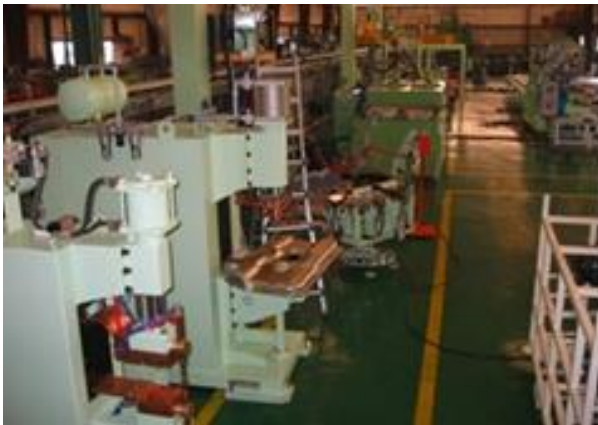
Fuel Tank welding and assembly line
