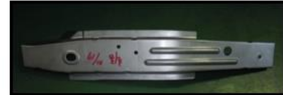
( HMC ) REINF-FR SIDE RR UPR,LH/RH Material : SGAF780 60/60
