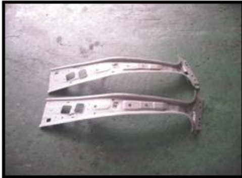
( GM ) CTR PLR INR L/RH Material : ST-S-270B2 1.0 mm
