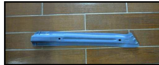
( GM ) RR SIDE DOOR IMPACT BEAM RH Material : 950YMS-AL60G60G
