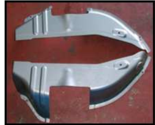
( GM ) WHEEL HOUSE Material : CR180B2 0.8 mm
