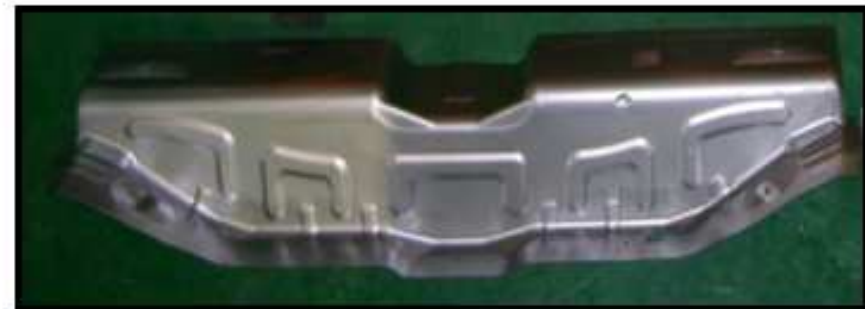
( GM ) EXTN FLR Material : SPRC440 1.0 mm
