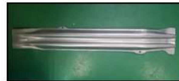
( HMC ) MBR FRT DOR IMPACT, L/RH Material : SPFC1180Y
