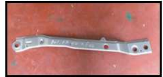
( PROTON ) SIDE MEMBER LOWER LH Material : DP590-P
