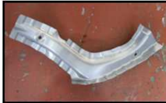
( PERODUA ) MBR,FR APRON TO COWL SIDE LWR FR RH Material : SCGA270D 1.2mm
