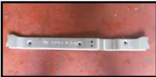
( PROTON ) CROSS MEMBER FRONT UPPER Material : DP590-P
