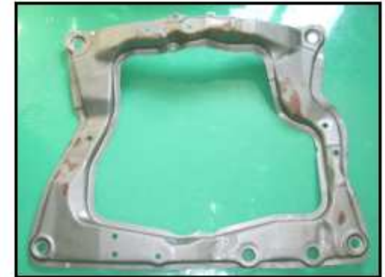
( HMC ) FRT FRAME Material : SPH-270D 1.6 mm
