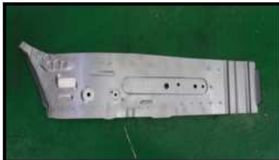
( PERODUA ) PLATE,FR SIDE MBR,OTR LH Material : SPCC 1.2mm
