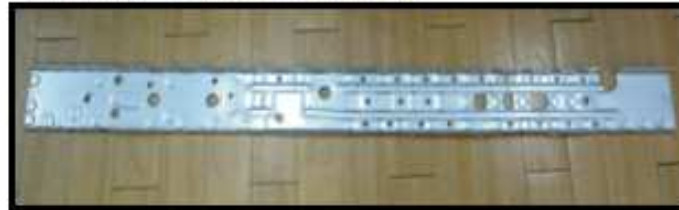
( GM ) REINFORCEMENT-RKR INR PNL LH/RH Material : CR980T/700Y-MP
