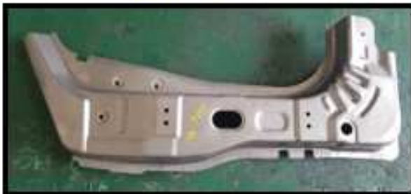
( POSCO ) A PILLAR LWR, LH Material : 1180TRIP
