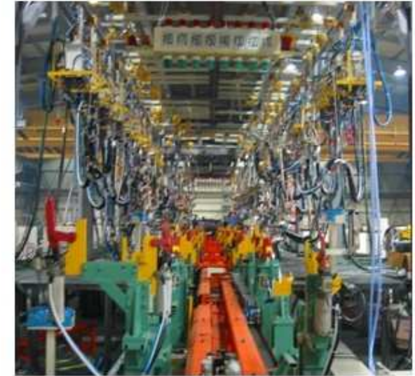
Door welding and assembly line
