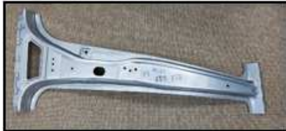
( POSCO ) B PILLER, LH Material : 1180TRIP
