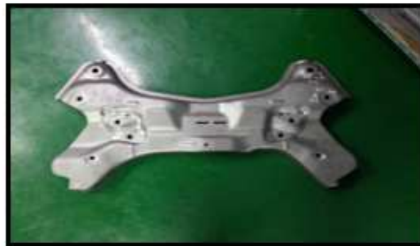
( HMC ) FRT CROSS MBR UPR Material : SGARC440 60/60 1.8 mm
