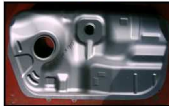
( KIA ) FUEL TANK UPR Material : SRNCEN 0.8 mm
