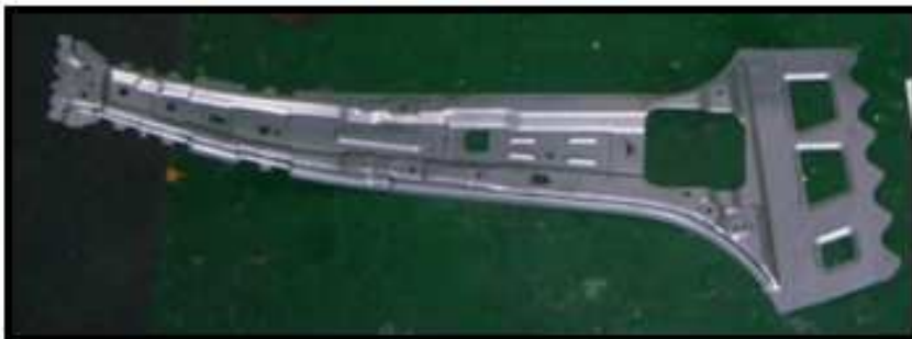
( GM ) CTR PLR L/RH Material : CR590/340Y-DP 1.4 mm
