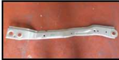
( PROTON ) SIDE MEMBER UPPER LH Material : DP590-P
