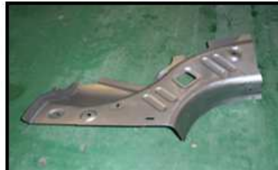
(PROTON ) PANEL REAR END LH Material : SPRC45 0.85mm
