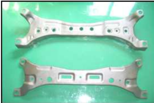
( HMC ) RR CROSS MBR Material : SAPH-38P 1.8 mm
