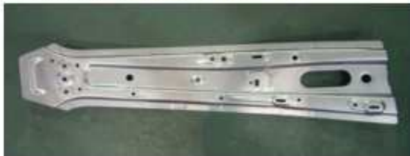
( GM ) CTR PLR LH/RH Material : CR980T/700Y-MP
