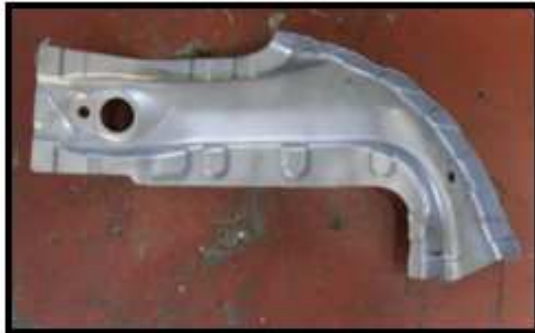
( PERODUA ) MBR,FR APRON TO COWL SIDE LWR FR LH Material : SCGA270D 1.2mm
