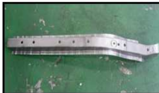
( PERODUA ) MEMBER,FR SIDE,RR RH Material : SPH440 1.2mm
